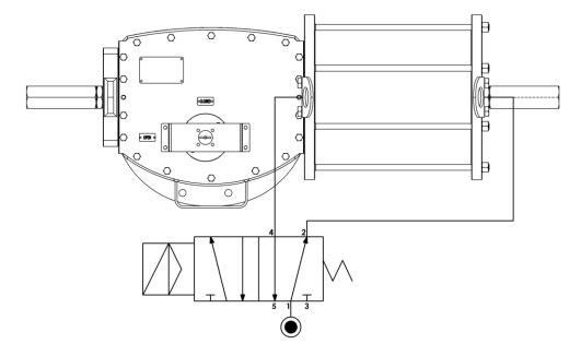
10. If possible, operate the actuator in order to check that it actuates smoothly the valve. Before this operation, verify that supply fluid composition, filtration and hydration correspond to the ranges for which the actuator was designed. In case of doubts please see the "Motive Energy" section on this manual or contact Actuatech technical department.
