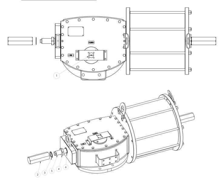
The setting of the open valve position is performed by adjusting the screw which is screwed into the housing closure flange:
