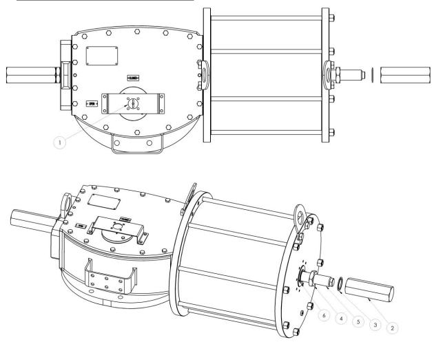
The setting of the closed valve position is performed by adjusting the screw which is inserted into the end flange of the pneumatic cylinder as follows:
