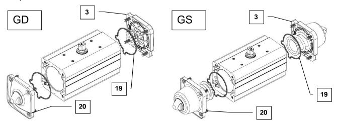
**Caution.** The Spring Return end caps cartridges (Parts N $^{\circ}$  3 + 18+24+19+23+22+21) are a safety device, where the preloaded spring is set to avoid the dangerous spring jumping. Do not release the screw (part N $^{\circ}$  21) to remove the spring from its seat, this operation must be done by Actuatech technician only.
