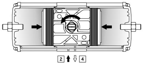
The port 2 is in connection with the cylinder side chambers, supplying the pressurised air in port 2 the standard Double Acting actuator drive shaft rotates counter clockwise to open, while the port 4 is in connection with the intermediate chamber and when pressurised the drive shaft rotates clockwise to close.
