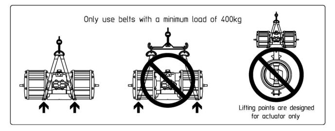
Before performing any installation operation, verify the actuator and valve conditions according to the safety notice above described.
